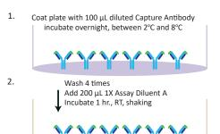
Wash 4 times Add 100 µL diluted standards and samples Incubate 2 hrs., RT, shaking
